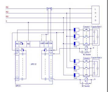
Quadrature Mode Method of Wiring (Basic & Expert Mode)
