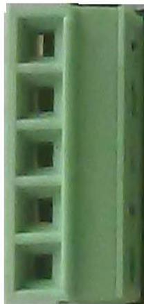
Fig: Connector for RS-232 and RS-485, towards the Top Left-Hand Side of the Cabinet.
